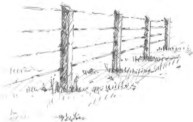
Wood post and wire
